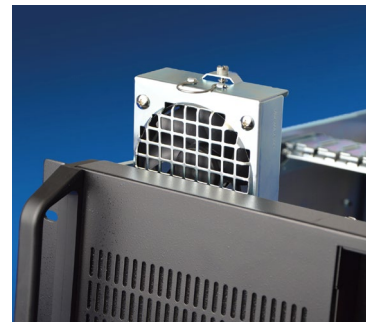
Easily replaceable fans inside the IPC 402
