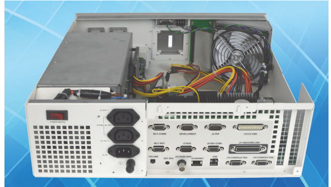
Rear view of the system with customer specific cut-outs for required interfaces
