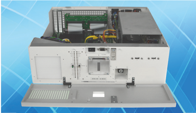
View of the open and custom designed front, top without cover
