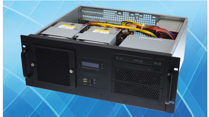
Front view of the open chassis, on the left with special bracket for the filter mat
