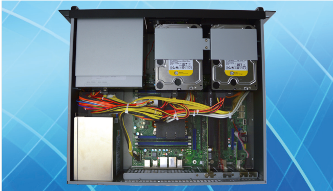
Insight into the completely assembled and wired high-end industrial PC
