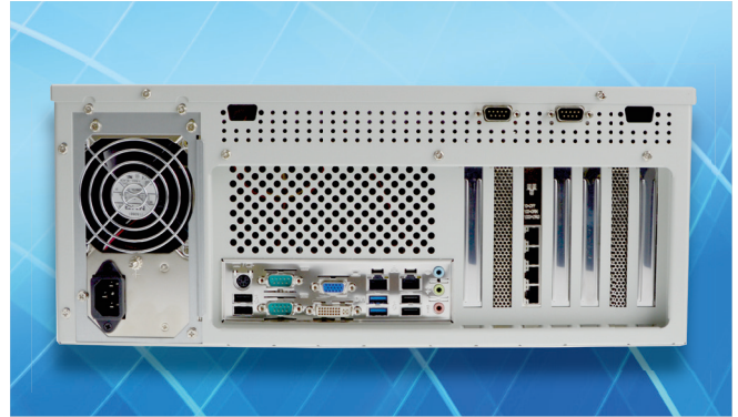
Rear view of the industrial PC with customer-specific cutouts for subsequent on-site retrofits by the customer
