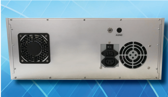
Rear view - with fan installation to the left and input for ATX power supply to the right
