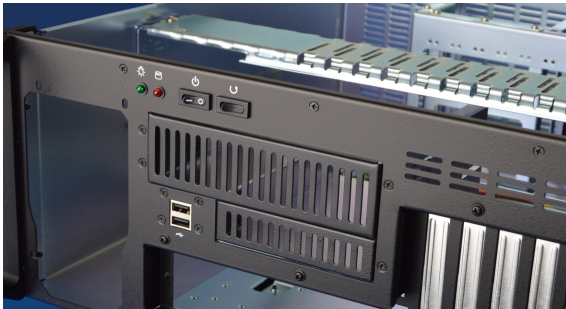
Drive bays, USB 2.0, power supply slot and controls are integrated into the front panel
