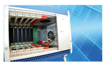
View of the inside of the system platform with VPX backplane and fan unit.
